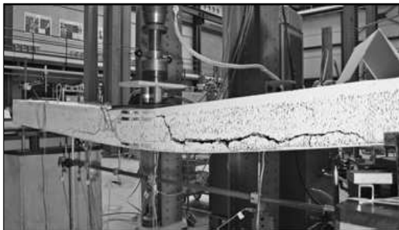
Typical failure of unbonded beam
